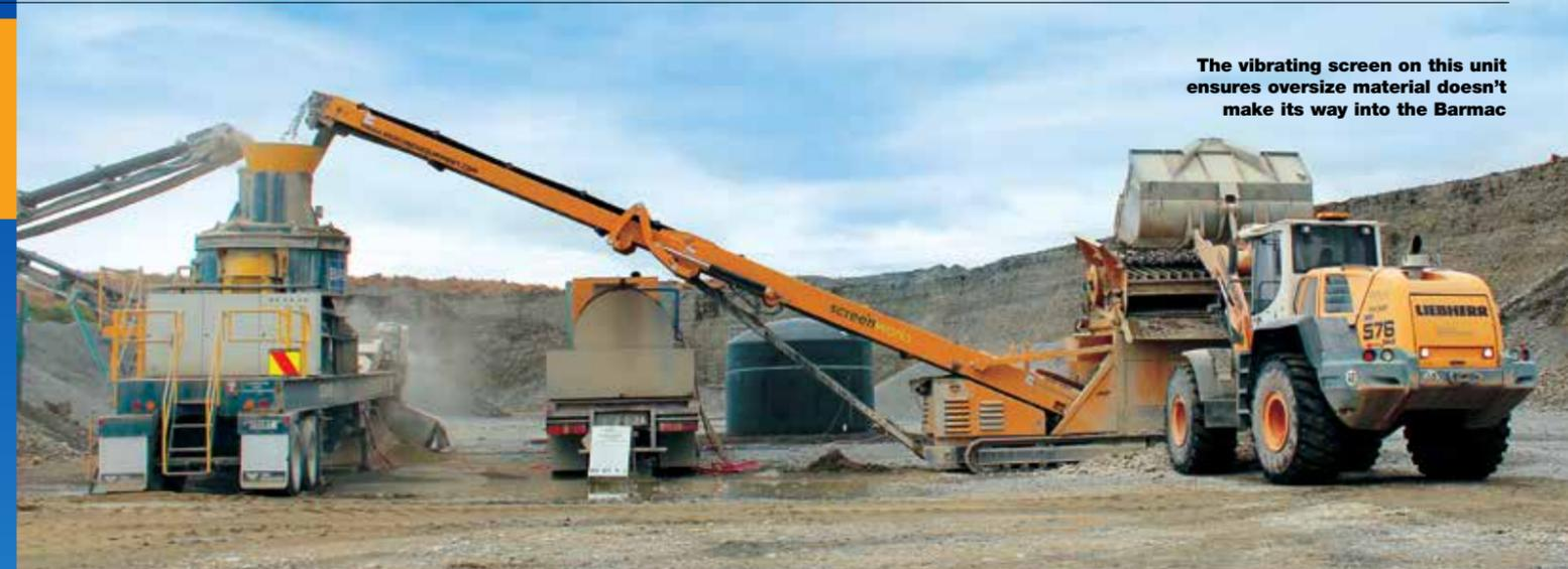
**The vibrating screen on this unit ensures oversize material doesn't make its way into the Barmac**
